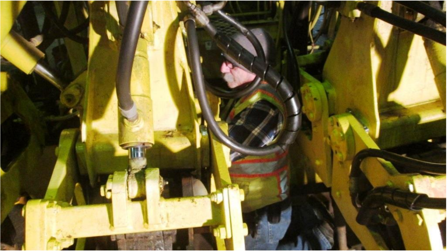
Joe installing the vibrator motor on one of the tamper's work-heads
